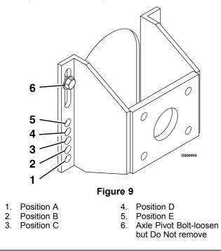
**Note:** The axle positions are in 1/2 inch (1.3 cm) increments and the large caster spacers are 1/2 inch (1.3 cm) thick. Therefore, by adjusting the same number of 1/2 inch (1.3 cm) caster spacers as
